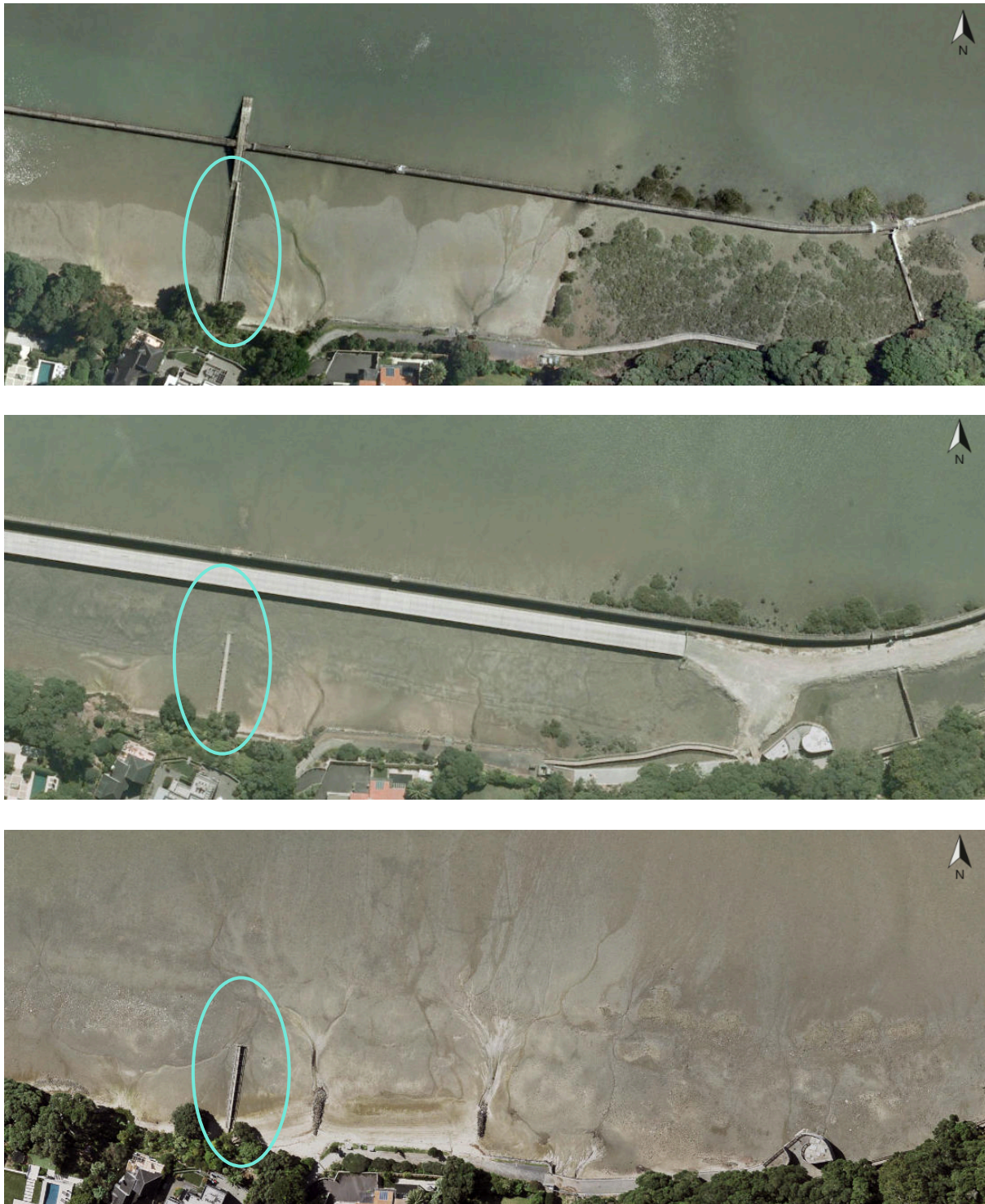
Figure 11: Series of aerial images (from top to bottom) 2008, 2010-11 and 2017 showing the Wilson's Beach Jetty (circled). Note in 2010-11, works have commenced with the removal of the main sewer line and shows that the extension over the line has been removed together with a section of the north end of the jetty. The 2017 image shows the jetty with no exposed sewer line (Auckland Council Geomaps).
